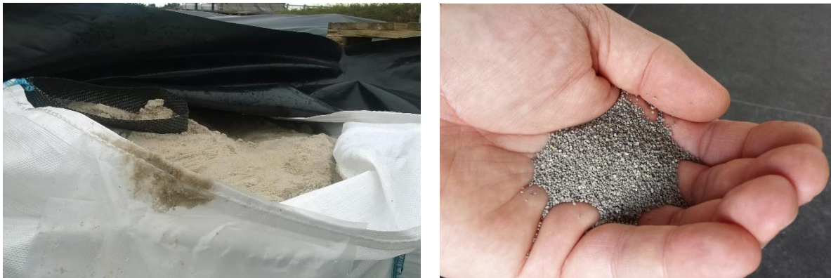
Figure 3.3. Pictures of struvite from the WWTP in Apeldoorn (left), which is used as raw material for the production of the fertiliser Physiostart P Plus bij Timac Agro (right).
