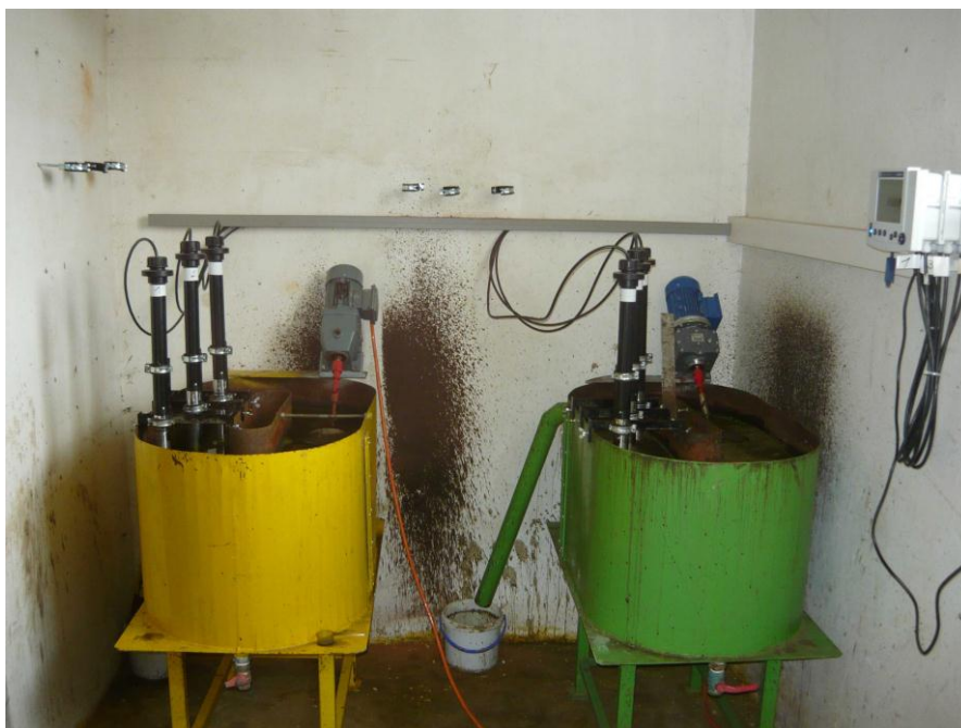
Figure 4.2. The two experimental units (GÜKON-Pilotfermenter) used to biologically acidify slurry and continually monitor pH, Eh, EC, and temperature.
