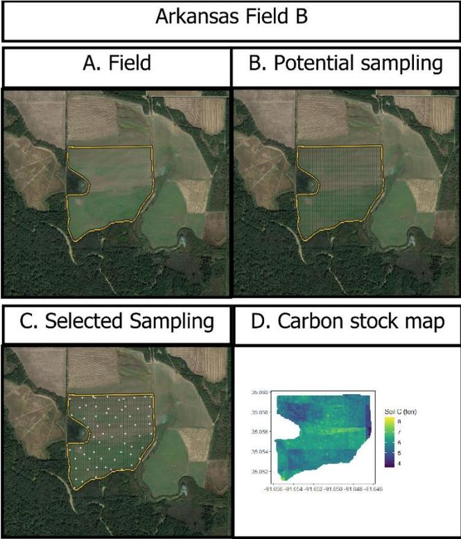
Figure 6-1. Visualisation cLHS sampling technique. Window A shows Field B in Arkansas, window B shows potential sampling locations, window C the selected sampling locations, and window D the resulting carbon stock estimates.
