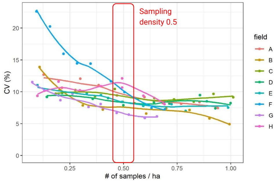
Figure 3-3. The coefficient of variation (CV%) in predicted field-level C stock versus the amount of samples per hectare taken. The CV is a measure of model precision, the lower the better. The CV levels off around 0.5 sample/ha, even for the smallest field (10 ha).
