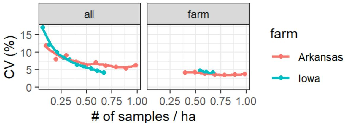
Figure 6-22. The Coefficient of Variation (CV, %) of the carbon stock for the two farms in Iowa and Arkansas. The CV of the carbon stock that uses data from the previous field campaigns (scenario “all”) reaches the threshold of 5% around a sampling density of 0.5 samples per ha.
