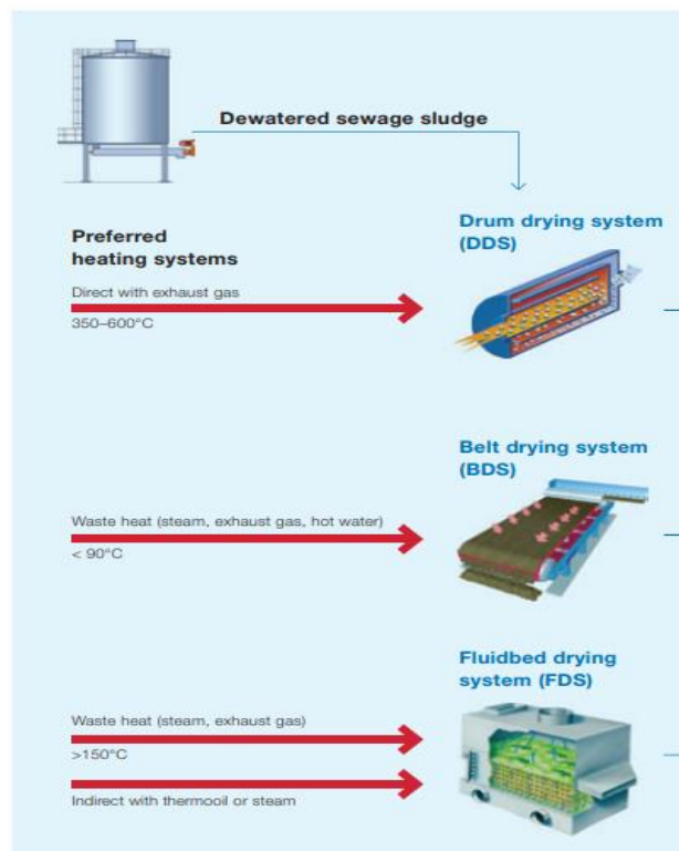
Figure 7. Three types of drying systems in use by Andritz Dryers based on temperatures and heat source (Andritz, 2012).
