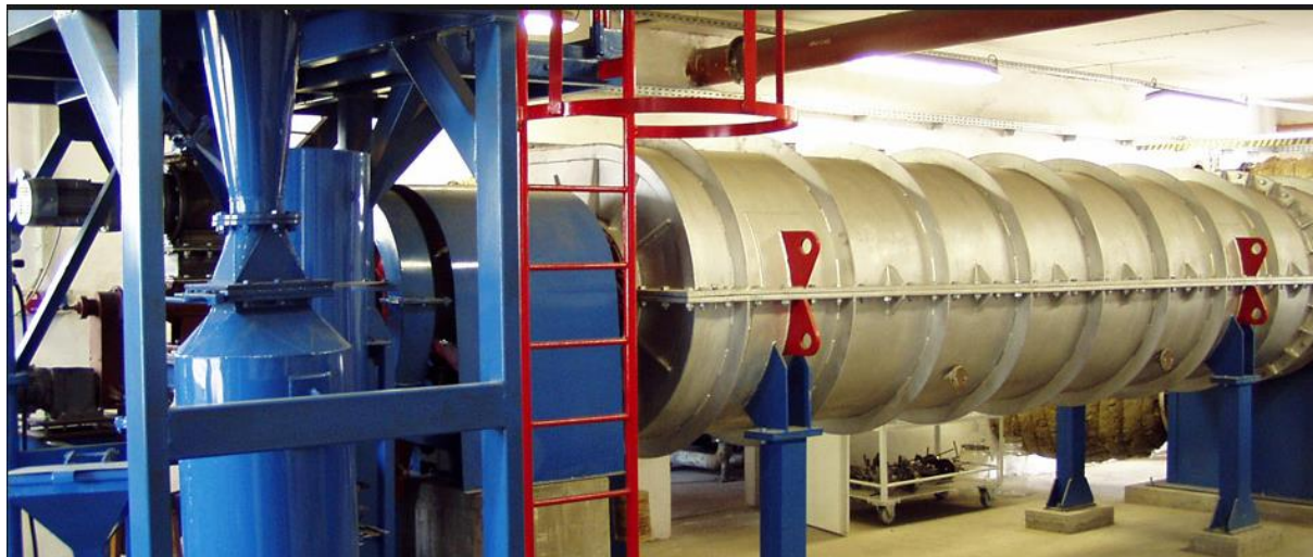
Figure 9. Pyrolysis reactor at Terra Humana (Terra Humana, n.d.)
