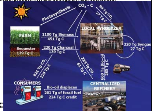
Fig. 1. The Charcoal Vision: A national system of distributed pyrolyzers for processing biomass into bio-oil and charcoal, with the bio-oil displacing fossil fuel and the charcoal being returned to the soil, could reduce U.S. demand for fossil oil by 25%, reduce U.S. C emissions by 10%, enhance soil and water quality, increase agricultural productivity, and strengthen rural economies.
